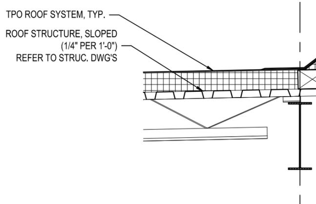
Figure 3: Section through penthouse roof. From 1/A4.09
