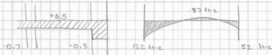
No beams (Interior Span) Short Direction
