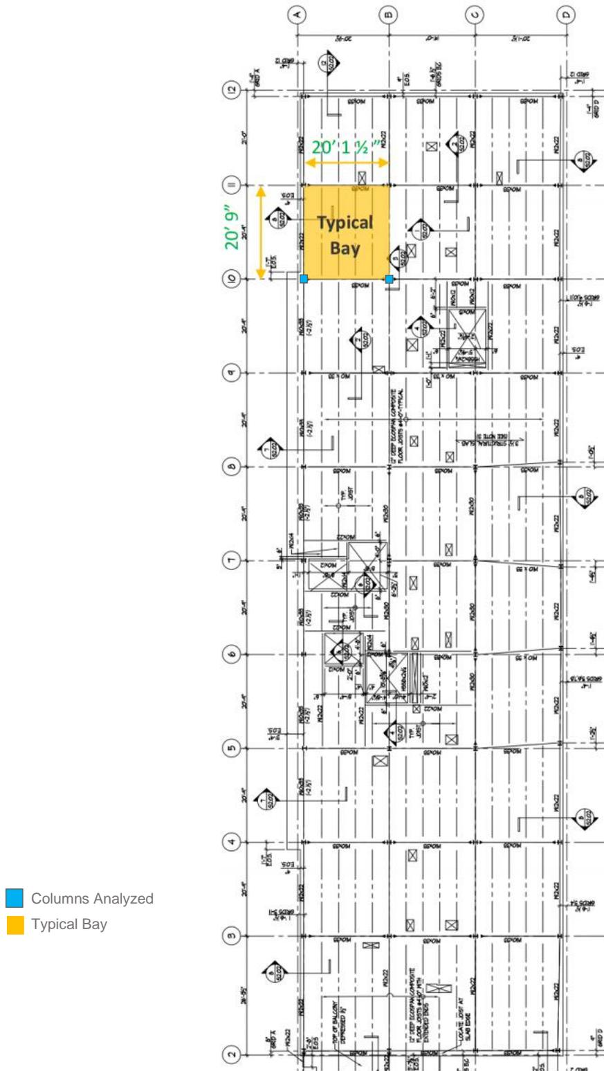
Figure 9: Typical Bay and Columns Analyzed for Gravity Loads, S1.07
