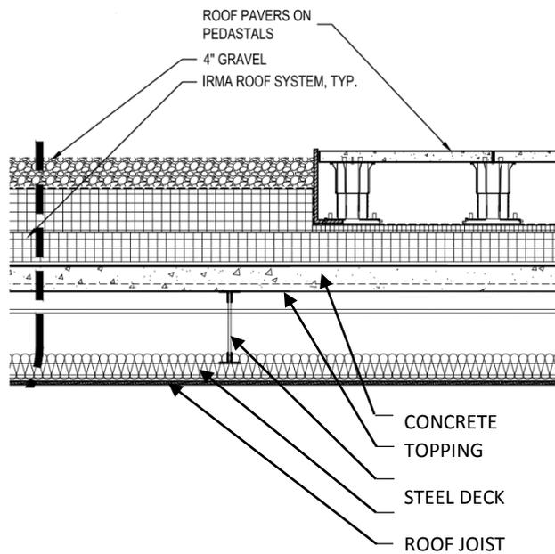
Figure 4: Section through roof at the 12<sup>th</sup> floor terrace level. From 3/A4.09.
