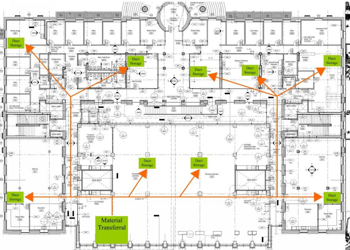
Figure 3 – Detail of the logistics plan showing the distribution of the ductwork to general locations of their installation
