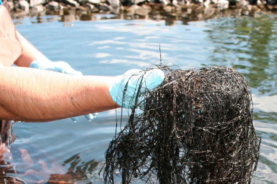
Biogenic manganese oxide-coated coir fiber collected from the coal mine drainage treatment system in Glasgow, Pennsylvania.
