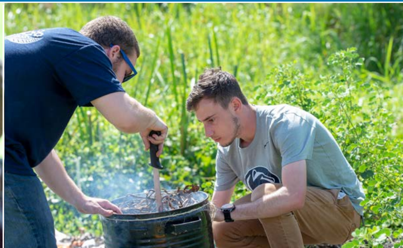
Members of GreenBriq carbonize dried water hyacinth, an invasive species on Lake Victoria, in the process of making briquettes for use as a sustainable fuel in cook stoves in the local village.
