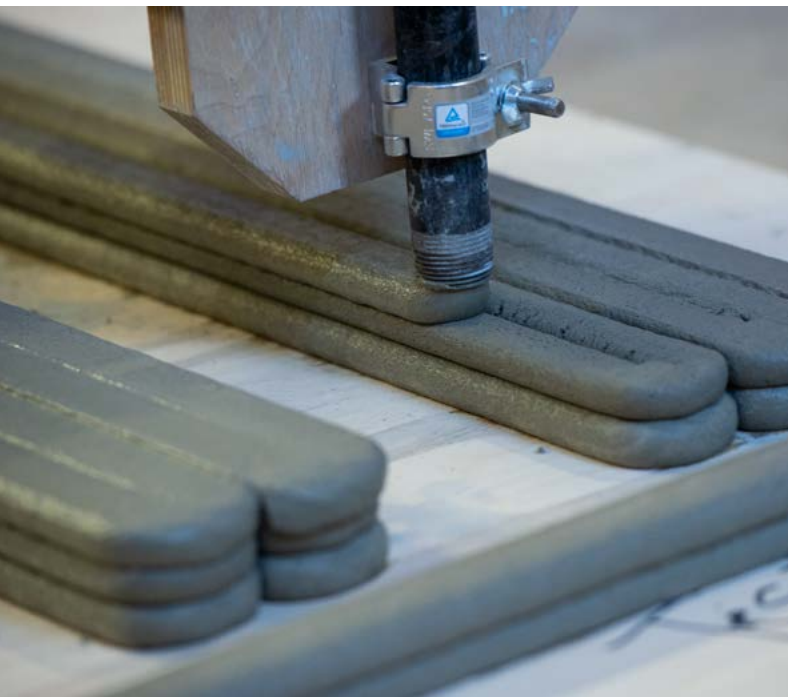
Printing tests to model material deformation during printing, from the work of architectural Ph.D. candidate Negar Ashrafi.
