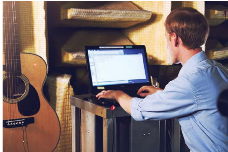
Micah Shepherd in the anechoic chamber demonstrating the testing used to determine the vibro-acoustic fingerprint for a Martin Guitar.
