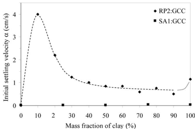
Figure 7. The effect of relative geometry on the initial settling velocity,  $\alpha$ , of dilute suspensions. The mixtures were prepared with the same carbonate GCC, but with different kaolinites: RP2, SA1.
