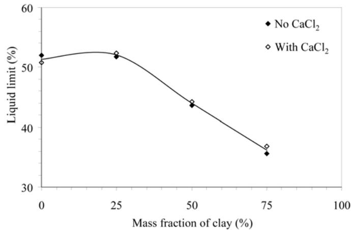
Figure 12. Controlling particle interaction through changes in surface chemistry and pore fluid. Liquid limit for Premier-PCC mixtures with and without CaCl<sub>2</sub>.
