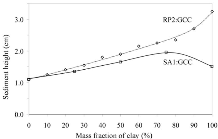
Figure 8. The effect of relative geometry on the 273 *H* sediment height of dilute suspensions. The mixtures were prepared with the same carbonate GCC, but with different kaolinites: RP2, SA1. The sediment height is determined at the sediment-suspension interface.
