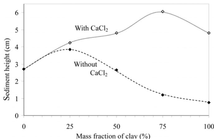
Figure 10. Controlling particle interaction through changes in surface chemistry and pore fluid. Final sediment height at 23 days for Premier-PCC mixtures with and without CaCl<sub>2</sub>.
