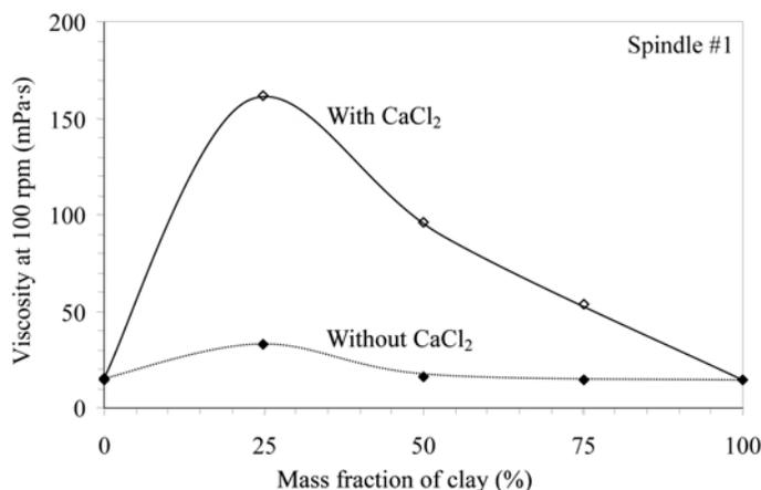
Figure 11. Controlling particle interaction through changes in surface chemistry and pore fluid. Viscosity at 100 rpm for Premier-PCC mixtures with and without CaCl<sub>2</sub>.
