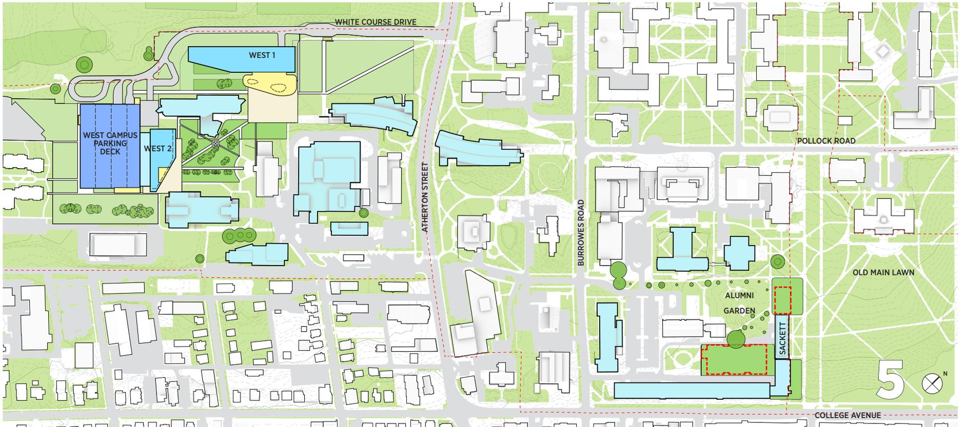
**Step 5** demolishes the Units and the North Wing of Sackett. Existing sewer and stormwater pipes run below the Units and will need to be relocated to run along the west side of Sackett and along the east end of Hammond to connect to the mains that run east along College Avenue. These sewer and stormwater pipes are temporary and will need to be relocated further west once Hammond has been demolished and construction of Core 1 begins.
