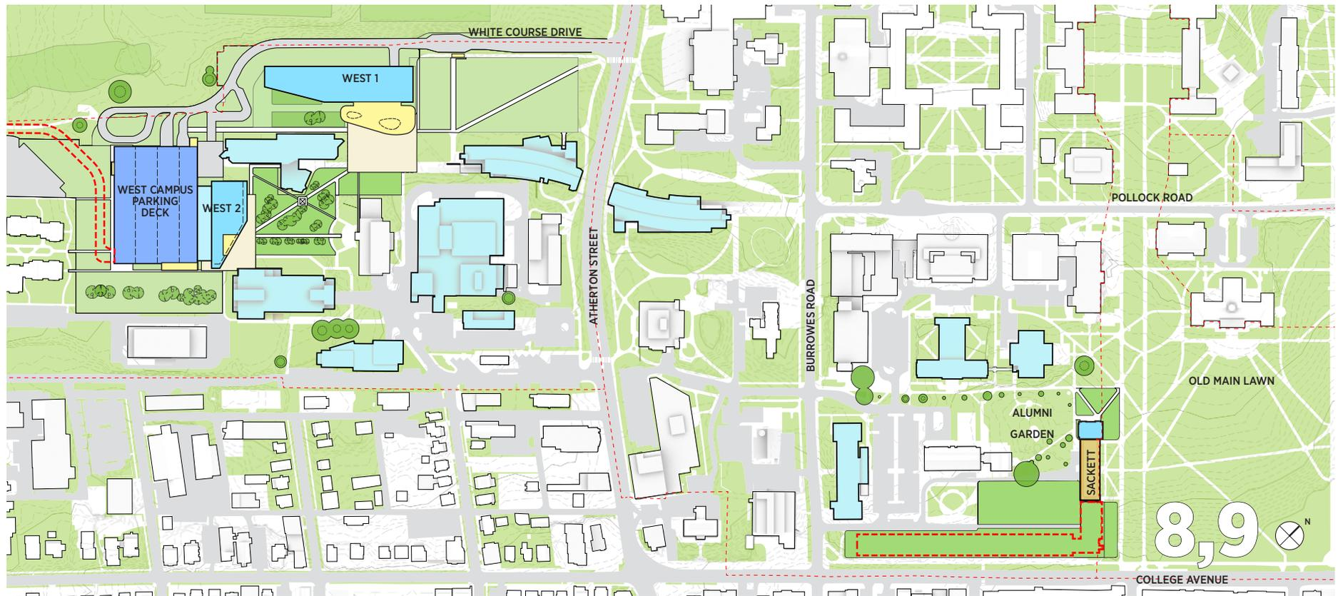
**Step 8** will demolish Hammond, the South Wing of Sackett, and Kunkle Lounge, including removal of the utility service laterals. The existing steam tunnel that runs below the sidewalk along College Avenue, south of Hammond, must be protected and not disturbed during building demolition. About 18,000 ASF of office space will require swing space at the end of Phase 1.
